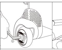
Turning anticlockwise on the left wheel screw for tighten the screw using tool ① and hold the nuts using tool ② inside the bag
