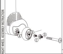
Install the (A) (B) (D) part through inside the frame wheels outside the bag
