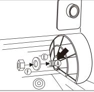
Put the (E) (F) part on screw (A) after the screw through inside the frame wheels inside the bag.
