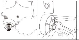
Turning anticlockwise on the right wheel screw for loosen the screw using tool ① and hold the nuts using tool ② inside the bag
