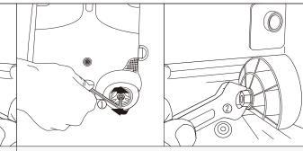
Turning clockwise on the left wheel screw for loosen the screw using tool ① and hold the nuts using tool ② inside the bag
