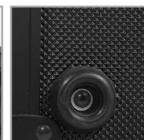
Rubber feet at the bottom for support in standing position
